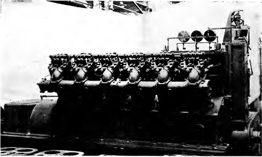
One of a pair of 300 b. h. p. Winton twin-six Diesel engines for the yacht "La Bell." The cylinders are 7\frac{1}{2} in. diameter by 9 in. stroke
